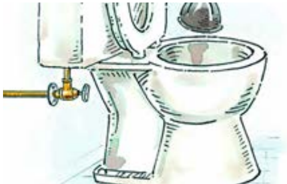
TOILET shutoff. This valve is usually on the cold-water supply located underneath the tank.
