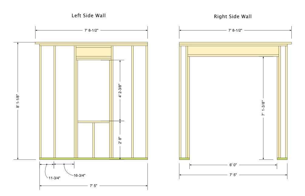
Figure E Posts and Front Beam
