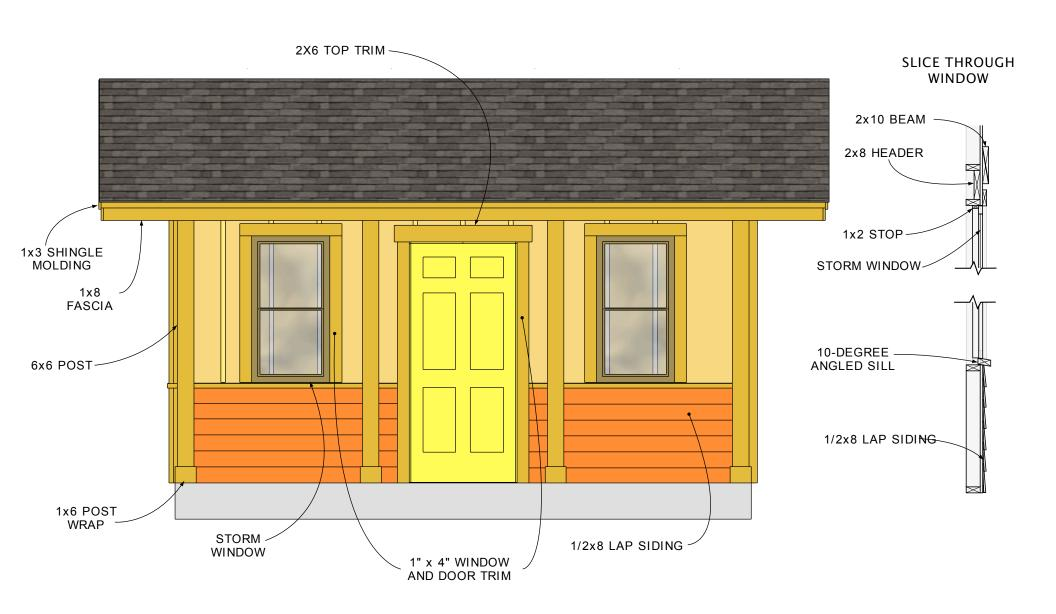
Figure Q End Wall Siding and Trim
